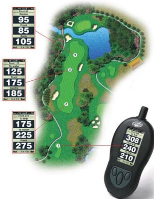
Caddy Maps For your Caddy to work on a particular course it needs to be loaded with a Caddy Map. A Caddy Map is a set of Latitude and Longitude reference points which represent the key hazard points of the hole and the Front, Centre & Back of the Green.
